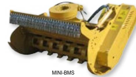
The MINI-BMS is the lightest forestry mulcher in the SEPPi range of excavator mounted mulchers. Its light weight makes it ideal for long excavator arms. This way the mulcher will reach even far off spaces.
