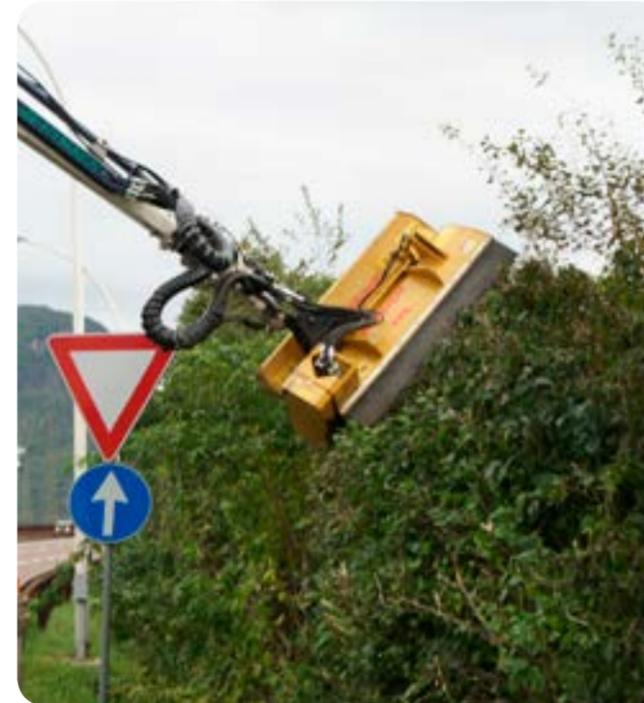
The excavator mounted mulchers come with hydraulic drive and have been made specifically for being mounted on excavator arms.
