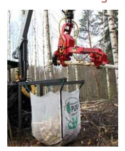
S23 guillotine is designed with decades of experience. Guillotine is strong, reliable and easy to maintain. Cutting blade can be mounted with splitting wedges to make 25-50 cm firewood directly after felling. Wedges are easy to mount and dismount with 3 bolts. Naarva firewood rack can be mounted to threepoint linkage of a tractor to hold a firewood bag. Firewood can be made directly to firewood bags after felling.
