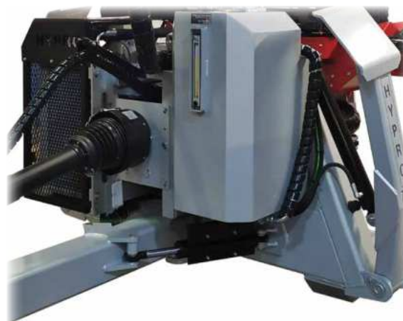
Articulated steering +/- 25° with double steering cylinders.
