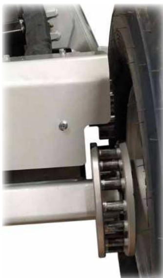
Articulated steering +/- 25° with double steering cylinders.
