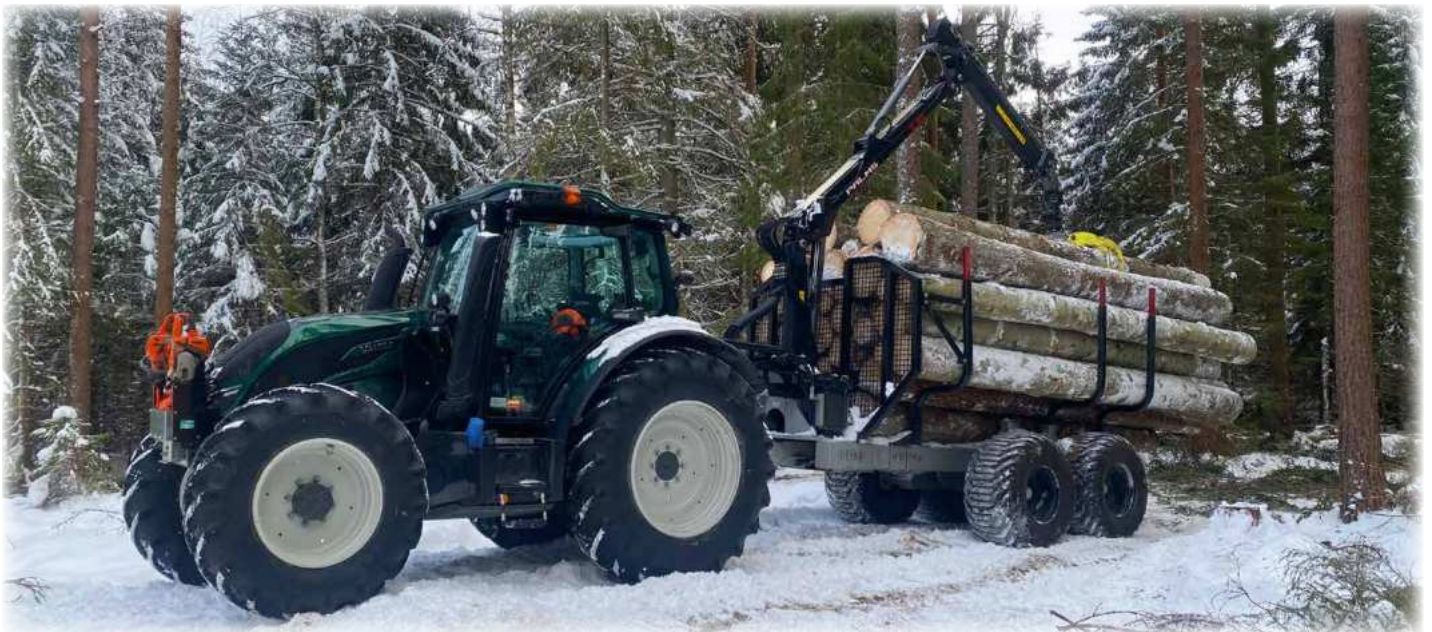
The loader in the picture is a Palms 5.85 with a maximum length of 8.5 m. We offer several different makes and crane lengths of up to 10m. The control system is our internally developed HYPRO+1 Canbus system.
