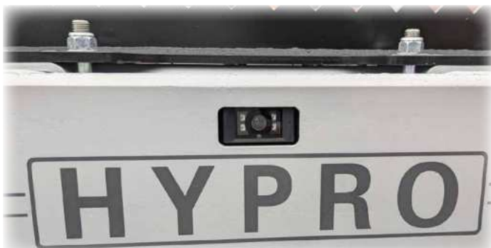
Wireless reversing camera is a popular optional extra on HV14. The camera is located in a well-protected position on the light board and provides a very good view behind the trailer.
