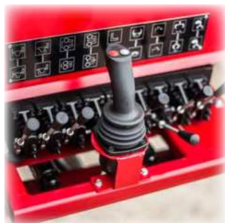
Automatic cross-cutting system with EHC-joystick on HYPRO 450 XL .
