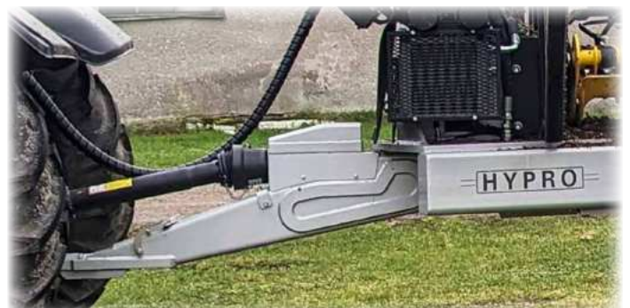
The trailer can be supplied without a hydraulic system, with an open pump hydraulic system or, as here in the picture, with 150L/min. load-sensing (LS) system.
