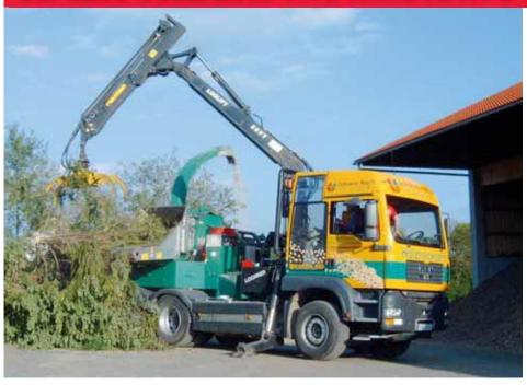
**As early as in the year 2004, Mus-Max and the company Lochner mounted the WT 9 wood chopping machine on a MAN truck.** It was the first to be driven directly by the truck engine. The original truck diesel engine ensures optimum cost-efficiency and can be used for driving or chopping operation alternatively.
