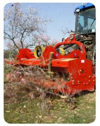
Certain crops produce very high quantities of prunings. This can cause big problems when it is time to mulch them. Burning is always bad for the environment. The MINIFORSTpick-up provides a perfect solution – picking up the prunings with a pick up reel at ground level and, if needed, reinforcing the feed into the machine with an optional top reel. The prunings are then processed within a screen to produce a fine and uniform mulch.
