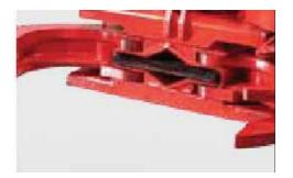
All Naarva felling heads are equipped with an efficient guillotine that cuts the wood with a single blade. The 12 mm thick blade is made of wear-resistant steel. Guillotine is maintenance free. Only maintenance required is greasing the joints. Guillotine is a safe and trouble free device for cutting trees.
