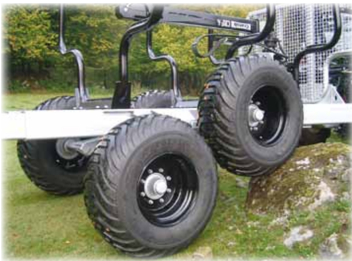
Bogie with 22° oscillate ability for good manoeuvre capacity at though terrain conditions.
