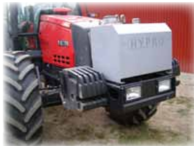
Hydraulic kit mounted in front.
