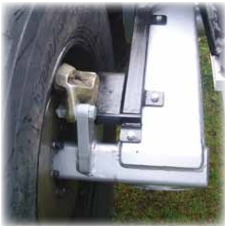
Hydraulic disc brakes on the bogie's front wheel pair and hydraulic drive on the rear wheel pair.
