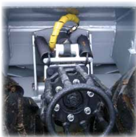
On the Hypro HV14 you have the option of choosing between robson drive or planetary gear. Hypro 4 WD rulldrift gives much higher drivepower and the driveunit is well protected
