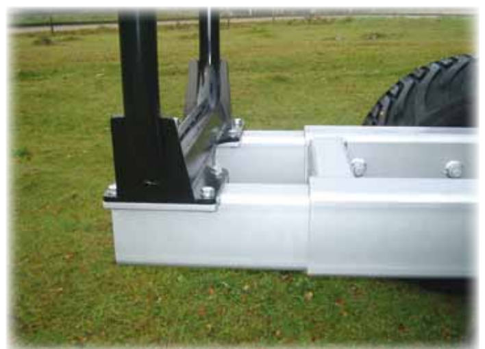
Additional bunk with manual telescopic length adjustment.
