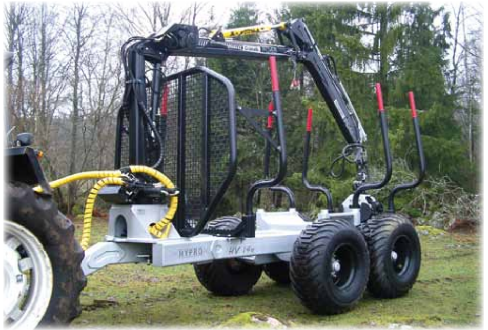
A Cranab FC45 with max lenght of 8,0 meters is used as crane.
