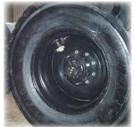
The drive device is placed in the rear wheel pair. Hydraulic motor drive via planetary gear generates very strong work force. With the drive activated, the hydraulic motor has automatic free rolling up to 40 km/h with the LS-system.
