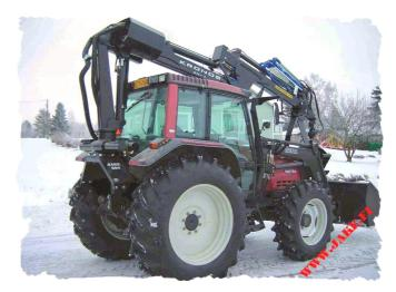
The JAKE 600 Mounting Kit makes using the tractor versatile because the crane mounted on the tractor can be combined with other devices and equipment connected with a 3-point linkage.
