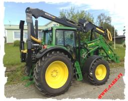
The JAKE 800 Mounting Kit makes using the tractor versatile because the crane mounted on the tractor can be combined with other devices and equipment connected with a 3-point linkage.
